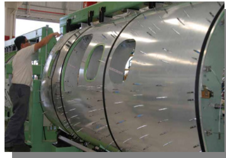
Phenom 100 central fuselage in the assembly process
