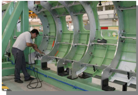
Phenom 100 central fuselage in the assembly process
